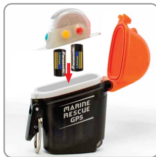
Insert two batteries (Must be installed with proper orientation +, - symbols)
